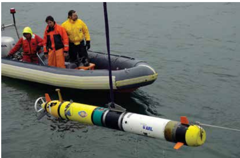
The IRAP system during a dockside dip test. The LF sensor is coiled and suspended at the vehicle mid-section. The HF sensor is located on the underside of the vehicle a couple of feet aft of the nose.
