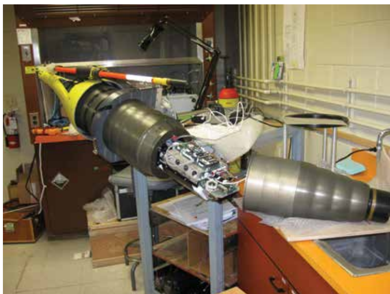
The PAM board installed in the Kongsberg Seaglider.
