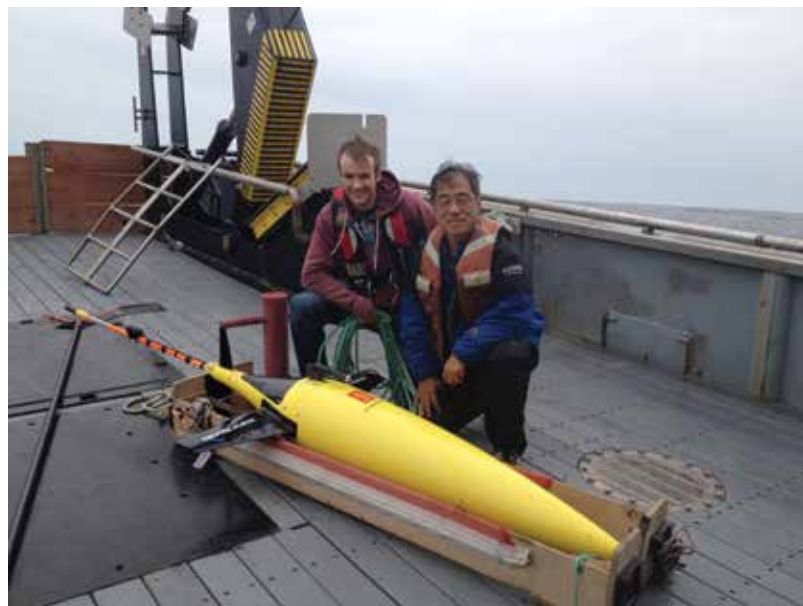
The Kongsberg Seaglider. The hydrophone is located on the orange antenna.
